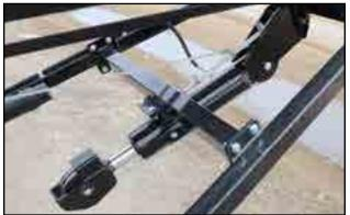
Fig 66 - Conveyor lift cylinder
