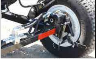
Fig 17 - Disengaged drive wheel
