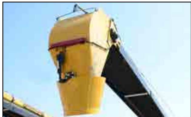
Fig 28 - Quad-swivel discharge spout and transport lights
