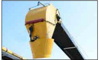
Fig 30 - Quad-swivel discharge spout and transport lights
