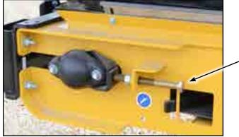
Fig 56 - Adjustment bolt on idler roller
