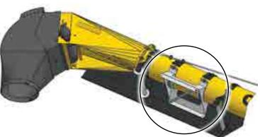
Fig 31 - Belt scraper after the discharge
