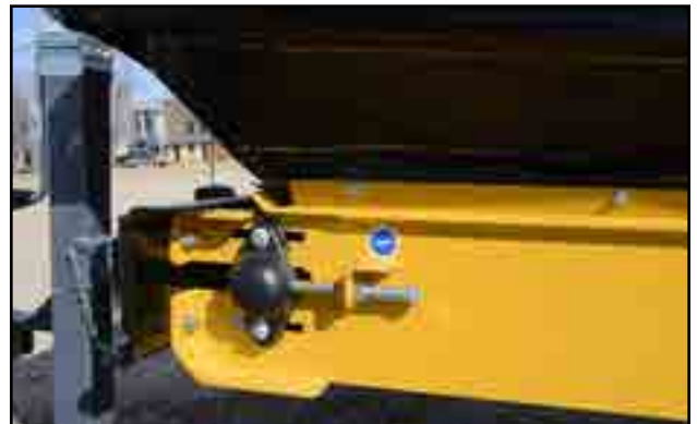
Fig 77 - Adjustment bolt at tail roller
