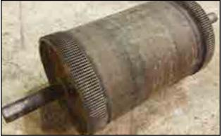
Fig 115 - Worn out drive roller
