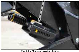
Fig 71 - Spring tension bolts
