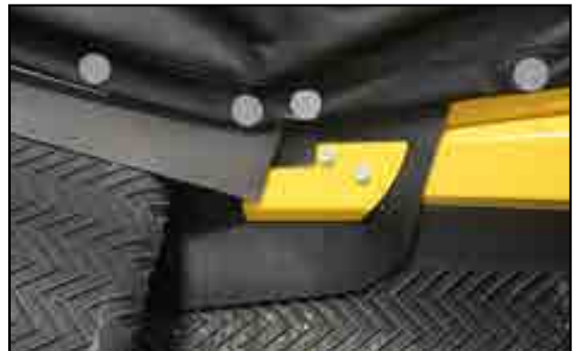
Fig 96 - Fasten flashing clamp
