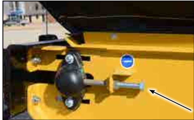
Fig 59 - Adjustment bolt on tail roller
