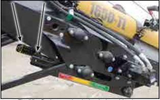
Fig 55 - Spring tension bolts, below drive box
