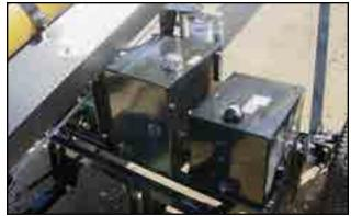
Fig 52 - Oil reservoir and fuel tank
