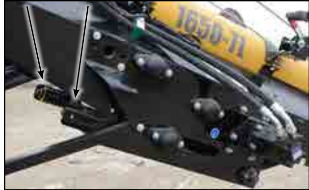
Fig 58 - Spring tension bolts, below drive box
