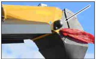
Fig 62 - Discharge roller bearing
