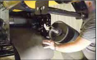
Fig 116 - New roller being installed
