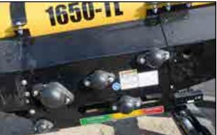
Fig 54 - Drive box roller bearings
