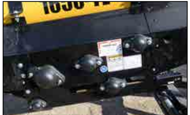
Fig 64 - Drive box roller bearings
