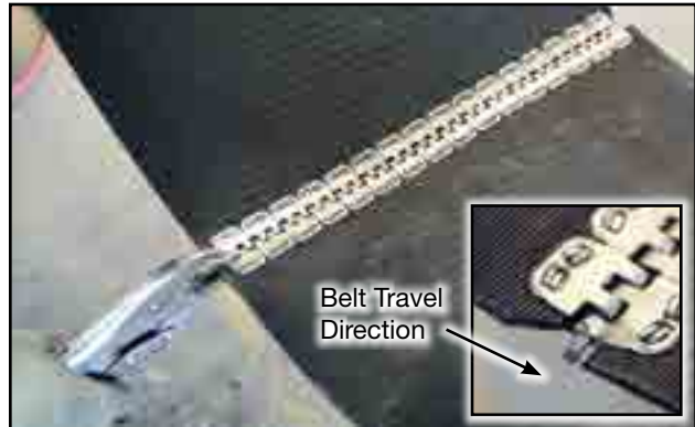
Fig 88 - Crimp lacing and taper belt corner
