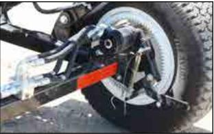
Fig 47 - Disengage drive wheels
