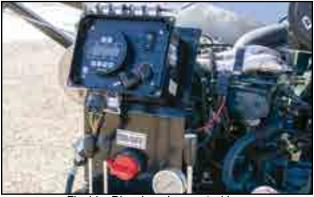
Fig 11 - Diesel engine control box
