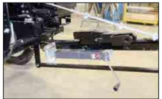
Fig 48 - Drawbar and jack storage plate
