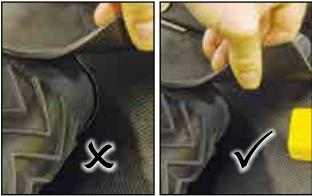
Fig 93 - Corner flashing must fit tight around the belt
