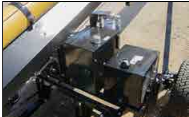
Fig 12 - Fuel tank and hydraulic reservoir
