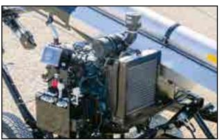
Fig 10 - Tier 4 diesel engine
