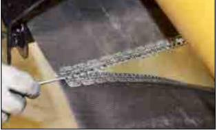
Fig 84 - Thread lacing cable
