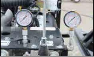
Fig 15 - Hydraulic pressure gauges
