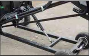
Fig 65 - Steering wheel lift cylinder
