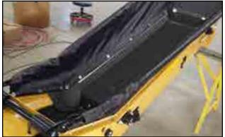
Fig 107 - Rubber flashing install
