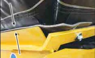
Fig 101 - Flashing flush with brackets
