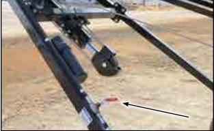
Fig 16 - Tube lift cylinder and ball valve
