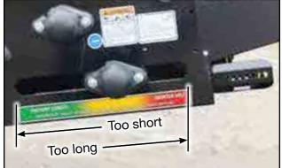
Fig 73 - "Slack Eliminator" roller. Belt length indication
