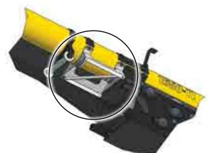
Fig 32 - Scraper before the drive box
