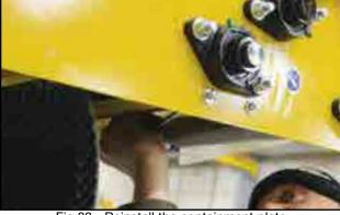
Fig 83 - Reinstall the containment plate
