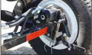
Fig 113 - Wheel ring gear and drive motor
