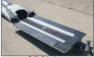
Fig 24 - Rail car hopper
