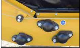
Fig 60 - Transition roller bearings
