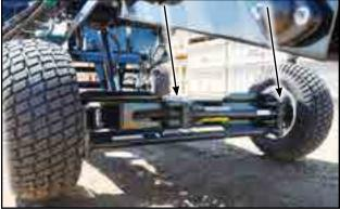
Fig 64 - Steering wheel axle bushings
