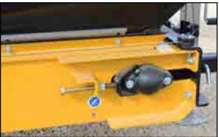
Fig 74 - Adjustment bolt at hopper idler roller
