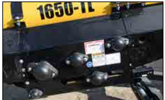
Fig 57 - Drive box roller bearings
