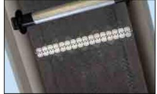
Fig 78 - Conveyor belt lacing
