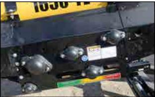
Fig 61 - Drive box roller bearings
