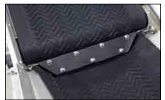
Fig 98 - Transition Flashing in place
