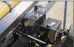
Fig 12 - Fuel tank and hydraulic reservoir
