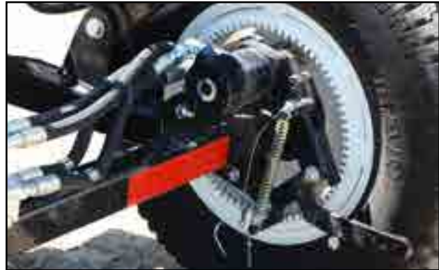
Fig 113 - Wheel ring gear and drive motor
