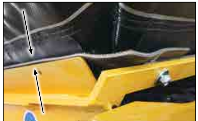
Fig 103 - Flashing flush with brackets
